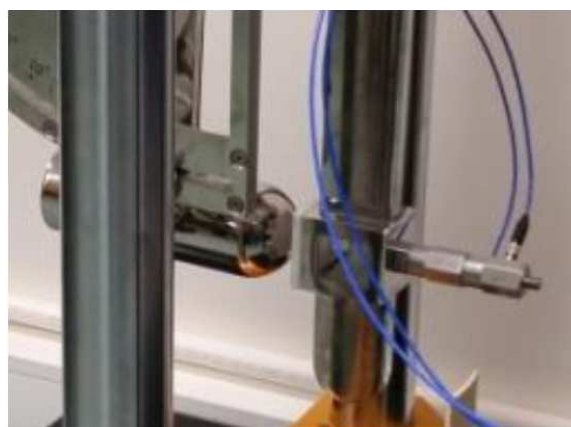
Fig. 1. Hammer and anvil pendulum of shock calibrator device, designed in TÜBİTAK UME.
