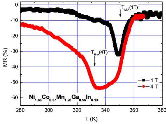
Fig. 5. Temperature dependence of MR effect in the Mn-rich Co- and In-doped alloy at field of 1 T and 4 T.
