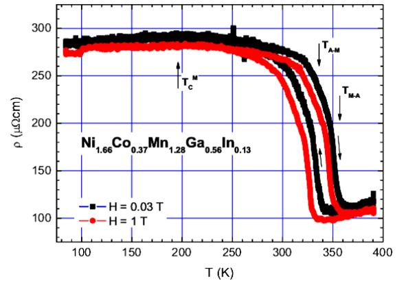
Fig. 4. Temperature dependence of resistivity of the Mn-rich, Co- and In-doped alloy at different magnetic field.
