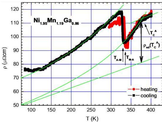
Fig. 2. Temperature dependence of resistivity of the Mn-rich alloy with fits (lines) by linear and quadratic polynomials.
