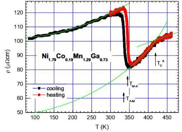
Fig. 3. Temperature dependence of resistivity of Co-doped alloy with fits (lines) by linear and quadratic polynomials.
