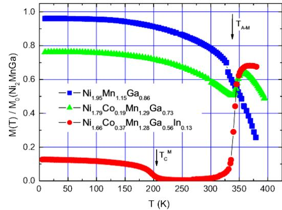
Fig. 1. Temperature dependence of magnetization of the selected alloys with respect to  $M(5 \text{ K})$  of the Ni<sub>2</sub>MnGa alloy.
