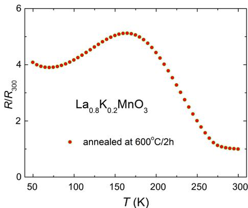
Fig. 6. Temperature dependence of the electrical resistance on the sample with rhombohedral crystal structure.
