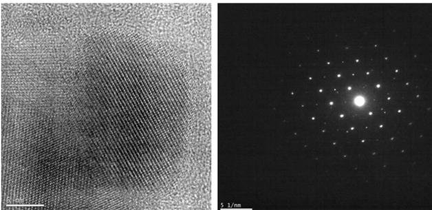
Fig. 2. HRTEM image of as prepared sample shows an individual particle. The white line represents the distance of 5 nm. Second photo shows the electron diffraction pattern.
