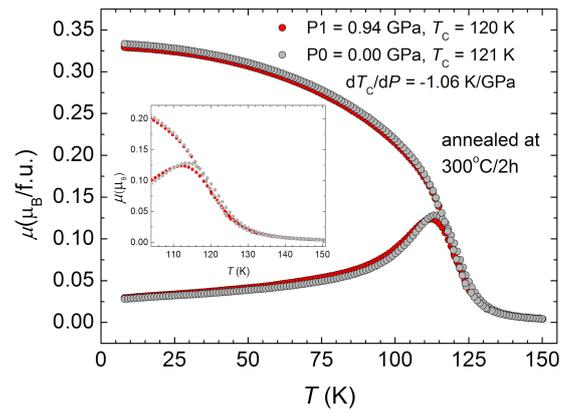
Fig. 3. ZFC and FC magnetization are shown at different pressures for sample with the orthorhombic crystal structure. The inset shows bifurcation and phase transition in detail.
