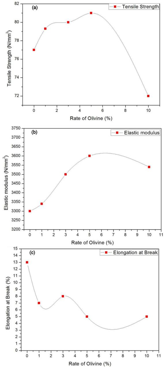
Fig. 1. Tensile test results for composites: (a) tensile strength, (b) elastic Modulus, (c) elongation at break.
