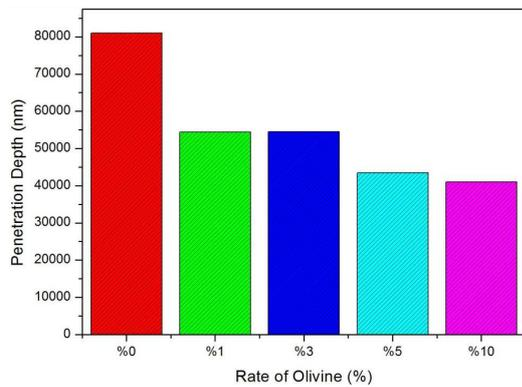
Fig. 2. Penetration depth of diamond tip in samples.
