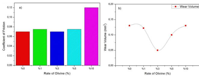
Fig. 3. Adhesive wear test results: (a) coefficient of friction, (b) wear volume.
