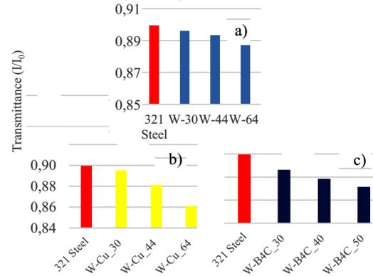
Fig. 2. Transmittance graph of tungsten (a), tungsten copper (b), and tungsten boron-carbide (c) coatings against Cs-137 gamma radioisotope.
