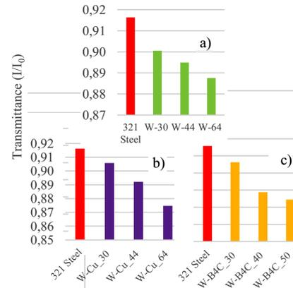
Fig. 3. Transmittance graph of tungsten (a), tungsten copper (b), and tungsten boron-carbide (c) coatings against Co-60 gamma radioisotope.
