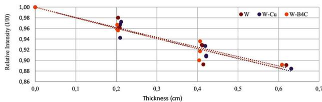
Fig. 4. Relative intensity — thickness graphs for tungsten, tungsten copper, and tungsten boron-carbide coatings on 321 steel substrate against Pu-Be neutron Howitzer (NH-3) neutron source.
