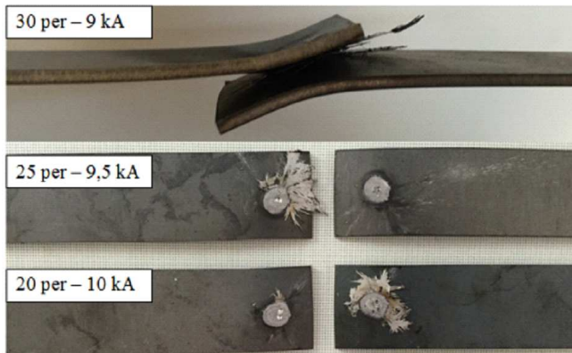
Fig. 4. Spurt out failure observed in weld nuggets.
