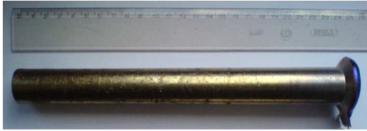
Fig. 1. A view of ingot of studied NiTi alloy.
