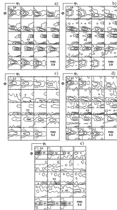
Fig. 2. Orientation distribution functions in sections \varphi_2 = \text{const} for \gamma -phase after 50% cold rolling (a) and ageing at 550^\circ\text{C} for: 30 min (b), 10 h (c), 24 h (d) and 100 h (e).
