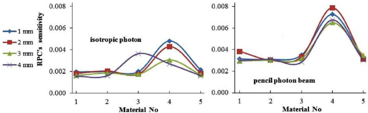
Fig. 3. Variation of RPC sensitivity depending on the type of the glass electrodes as calculated by FLUKA for isotropic and pencil photon beam.
