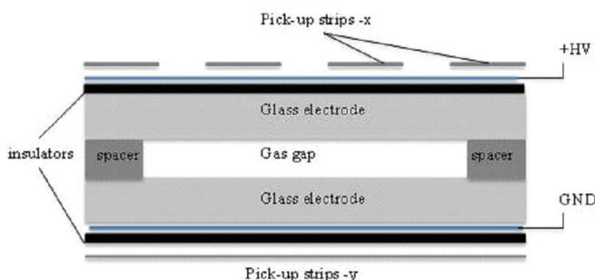
Fig. 1. The schematic illustration of typical RPC design.
