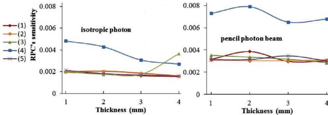
Fig. 2. Variation of RPC sensitivity with thickness of the five different electrode materials calculated by FLUKA for isotropic and pencil photon beam.
