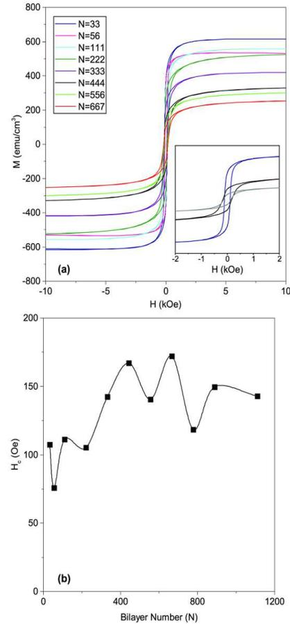
Fig. 2. (a) Hysteresis curves of  $N[\text{Co}(8 \text{ nm})/\text{Cu}(1 \text{ nm})]$  multilayers deposited with different bilayer number ( $N$ ), (b) coercivity ( $H_c$ ) values of the multilayers.
