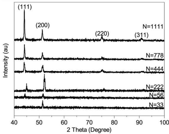
Fig. 1. XRD patterns of multilayers with  $N[\text{Co}(8 \text{ nm})/\text{Cu}(1 \text{ nm})]$  as a function of bilayer number  $N$ .
