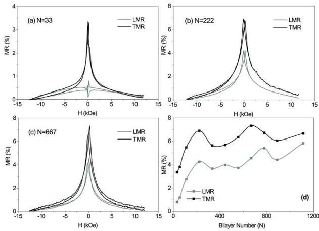
Fig. 3. TMR and LMR curves of multilayer having (a)  $N = 33$ , (b)  $N = 222$ , (c)  $N = 667$ , (d) variation of the GMR in  $N[\text{Co}(8 \text{ nm})/\text{Cu}(1 \text{ nm})]$  multilayers with bilayer number.
