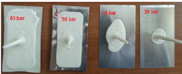
Fig. 2. The formability of the Al plates tested at different values of the injection pressure.
