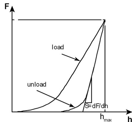
Fig. 4. Typical load-displacement curve used for calculation of the Young modulus [16].
