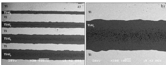
Fig. 2. SEM micrograph of laminated composites produced at 700 °C and 7.5h. (a) 30X, (b) 100X magnification.
