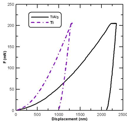
Fig. 5. Nano-indentation curve for MIL composite sintered at 700 °C and 7.5 h.
