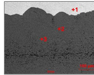
Fig. 3. SEM-EDS analyses of laminated composites produced at 700 °C and 7.5 h.
