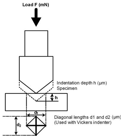
Fig. 1. Vickers type indenter.
