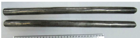
Fig. 2. View of UFG samples after ECAP at 160 °C and additional extrusion.
