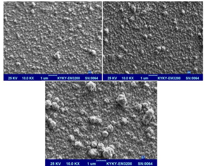
Fig. 6. SEM images of the ZnO thin films deposited at various glass substrate temperatures.
