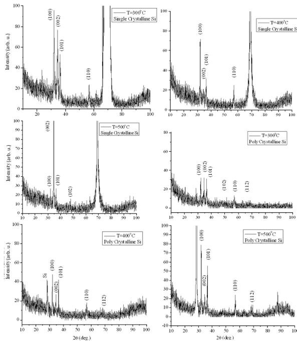
Fig. 5. XRD patterns of the ZnO layers grown on single and polycrystalline Si at three substrate temperatures of 300, 400 and 500 °C.
