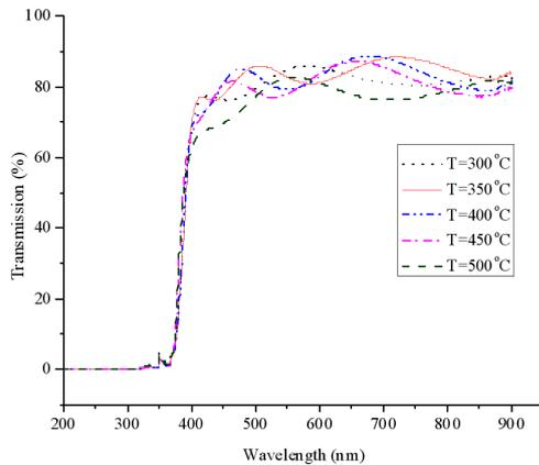
Fig. 7. Transmission spectra of ZnO thin films at different substrate temperatures.
