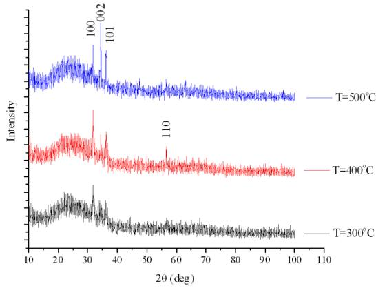
Fig. 3. XRD patterns of the ZnO layers grown on glass substrate at different deposition temperature.
