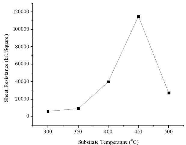
Fig. 1. Changes of sheet resistance versus deposition temperature.
