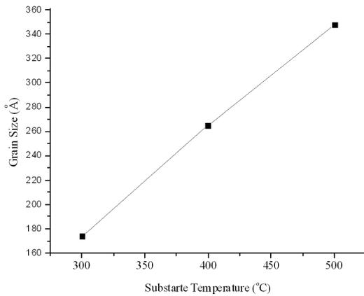
Fig. 4. Changes of grain size as a result of temperature increase.
