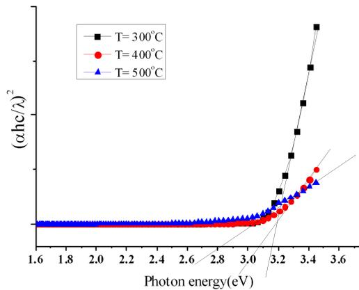
Fig. 8. Optical band gap of ZnO thin films at substrate temperature of 300, 400, 500 °C.
