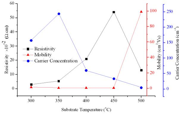
Fig. 2. Changes of electrical parameters such as resistivity, carrier concentration and mobility versus deposition temperature.
