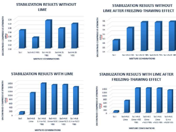
Fig. 3. Unconfined compressive strength of test specimens.
