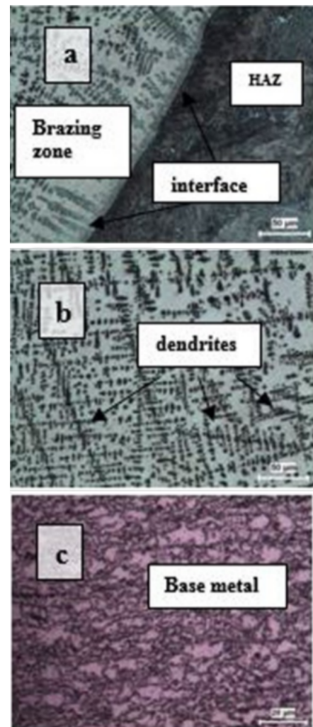
Fig. 2. MIG-Brazed TRIP 800 Microstructures, (a) interface, (b) braze, (c) base metal.
