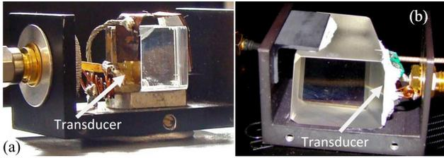
Fig. 1. (a) Acousto-optic deflector and (b) tunable filter on the base of paratellurite crystals under testing (cover removed).
