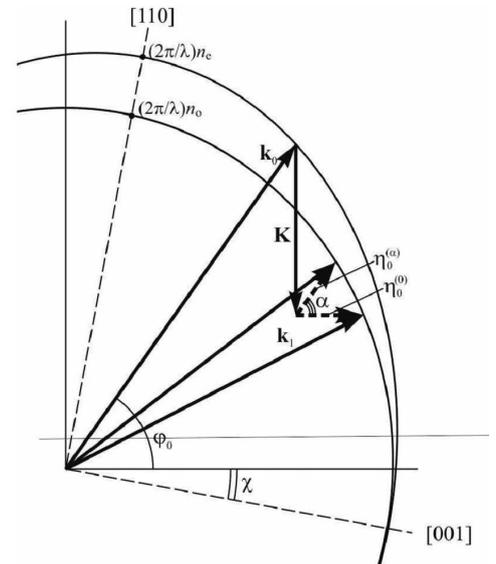
Fig. 3. Wave vector diagram illustrating the case, when the acoustic walk-off does not influence AO characteristics.
