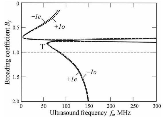
Fig. 2. Broadening coefficients as functions of acoustic frequency: +1o — diffraction of an o-wave into +1st order; +1e — diffraction of an e-wave into +1st order; -1o — diffraction of an o-wave into -1st order; -1e — diffraction of an e-wave into -1st order.
