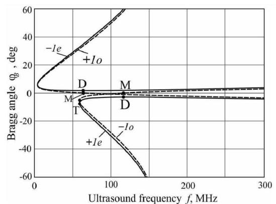
Fig. 1. Frequency dependence of Bragg angles in the case of anisotropic diffraction in paratellurite crystal: +1o — diffraction of an o-wave into +1st order; +1e — diffraction of an e-wave into +1st order; -1o — diffraction of an o-wave into -1st order; -1e — diffraction of an e-wave into -1st order.
