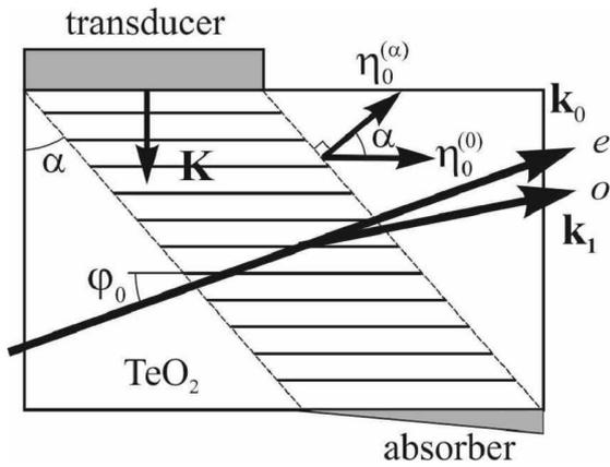
Fig. 4. Geometry of light and sound beams interaction in the paratellurite cell.
