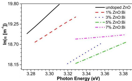
Fig. 2. Spectral dependences of logarithm of absorption coefficient for ZnO and ZnO:Bi films as a function of defects (Urbach plots).
