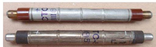
Fig. 1. Geiger counter STS-5 detector used in X-ray radiometer DP-66M.
