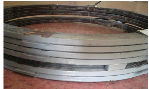
Fig. 3. Six coils of the real winding used for modeling, with visible axial shift.
