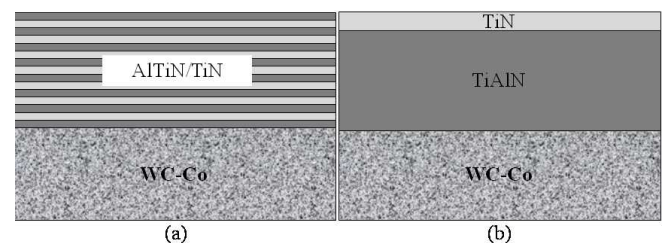
Fig. 1. Layer structure of the coatings: (a) nl-AlTiN/TiN, (b) commercial TiN/TiAlN coating.
