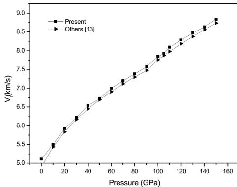
Fig. 6. Variation of the longitudinal elastic wave velocity ( $v_l$ ) with pressure.
