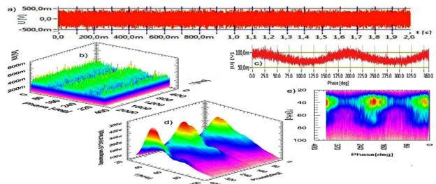
Fig. 5. Introductory description of the AE signal recorded at selected measuring point of the transformer (measuring line 1, measuring point 2): (a) impulse, (b) phase-time characteristic, (c) averaging phase characteristic, (d), (e) averaging STFT spectrograms, ADC = -9.70 (file T1B02(2).BIN, band of 100–200 kHz).
