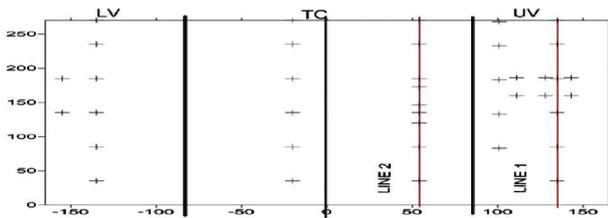
Fig. 1. Positions of measuring points at lateral walls of the tested transformer.
