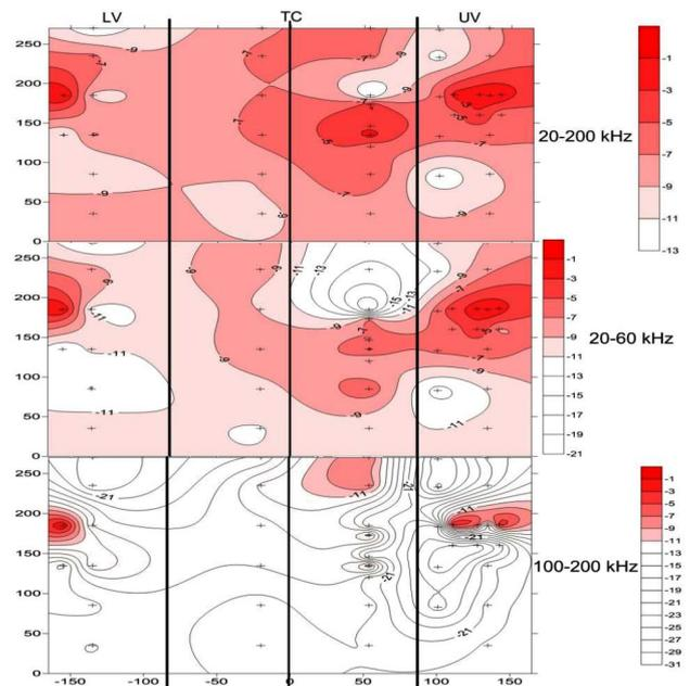
Fig. 2. Maps of ADC descriptor on lateral walls of the transformer tank within chosen frequency bands. Tank dimensions ( $X$ ;  $Y$ ) in cm:  $X$  — running position along the transformer tank, 0 — the center of the tap changer, positive  $X$  values — part of the tank from the side of the upper voltage, negative  $X$  values — part of the tank from the side of the lower voltage,  $Y$  — running height on the transformer tank, + — measuring points.
