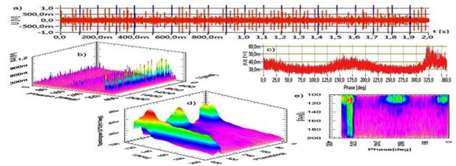
Fig. 4. Introductory description of the AE signal recorded at selected measuring point of the transformer (measuring line 1, measuring point 4): (a) impulse, (b) phase-time characteristic, (c) averaging phase characteristic, (d), (e) averaging STFT spectrograms, ADC = -3.06 (file T1G02(2).BIN, band of 20–100 kHz).
