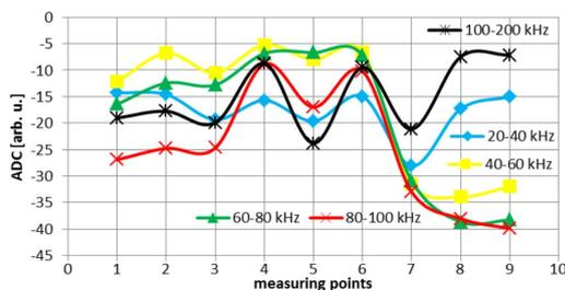
Fig. 6. Diagram of ADC descriptor values within chosen frequency bands from succeeding measuring points at line 2 (numeration of measuring points from the bottom of the line).
