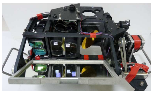
Fig. 1. Picture of the reflectance profilometer head.
