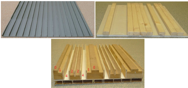
Fig. 2. Structures used to compare the space method and the boundary method. CDW - wells with constant depth; MLS - wells with maximum length sequence-based depths, QRD - with well depths determined by the quadratic residue series.
