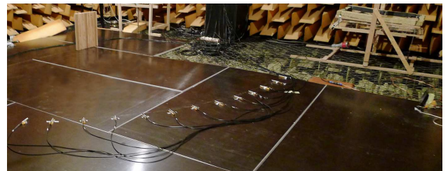
Fig. 1. A measurement set-up for determining the directional diffusion coefficient by means of the boundary method.
