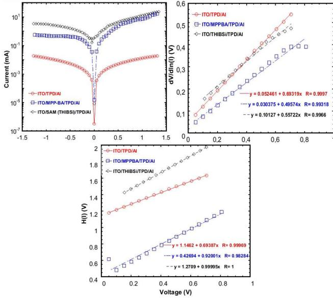
Fig. 3.  $I$ - $V$  characteristics of fabricated ITO/TPD/Al, ITO/MPPBA/TPD/Al, ITO/THIBSi/TPD/Al and devices.
