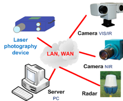
Fig. 1. Demonstrator of LPS hardware configuration.
