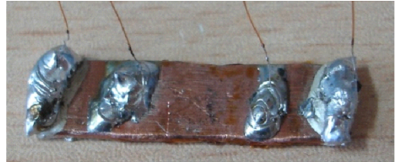
Fig. 1. Current and voltage contacts of MgB 2 /Fe/Cu multifilamentary tape.
