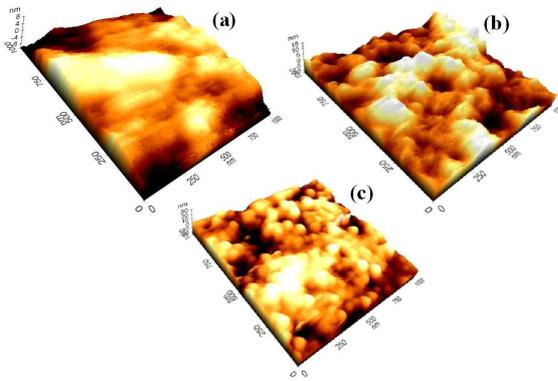
Fig. 2. AFM micrographs of the deposited  $\text{Fe}_{36}\text{Co}_{36}\text{B}_{19.2}\text{Si}_{4.8}\text{Mo}_2\text{W}_2$  thin films prepared by TVA for different thicknesses: (a) 200 nm, (b) 240 nm, (c) 260 nm.
