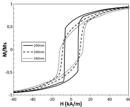
Fig. 3. The bulk hysteresis loop of  $\text{Fe}_{36}\text{Co}_{36}\text{B}_{19.2}\text{Si}_{4.8}\text{Mo}_2\text{W}_2$  amorphous films prepared by TVA for different thicknesses.
