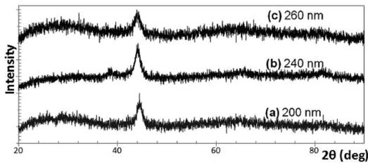
Fig. 1. Characteristic XRD patterns of the deposited  $\text{Fe}_{36}\text{Co}_{36}\text{B}_{19.2}\text{Si}_{4.8}\text{Mo}_2\text{W}_2$  thin films prepared by TVA for different thicknesses: (a) 200 nm, (b) 240 nm, (c) 260 nm.
