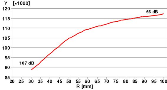
Fig. 7. Impact of the transition radius  $R$  on SPL.
