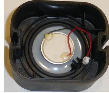
Fig. 3. Transducer mounted in the housing.
