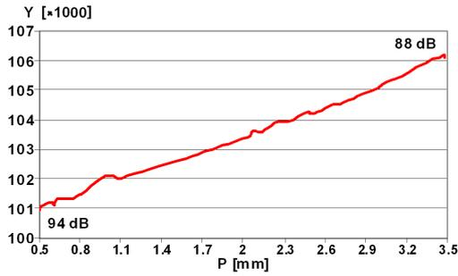
Fig. 6. Influence of fixing radius  $P$  on SPL.
