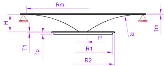
Fig. 1. Driver unit siren — the parameters considered.
