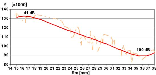
Fig. 8. Effect of the radius  $R_m$  on the level of SPL.
