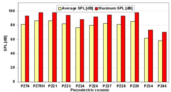
Fig. 4. Influence of the selected ceramics on the sound pressure level.
