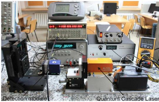
Fig. 7. Laboratory setup to measure optical power of the lasers.
