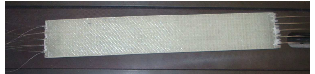
Fig. 2. Composite material sample with set of HB optical fibers embedded inside.
