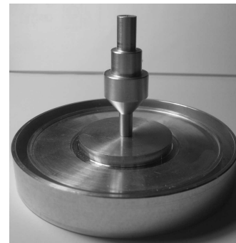
Fig. 4. Realization of modified flat sub-reflector.
