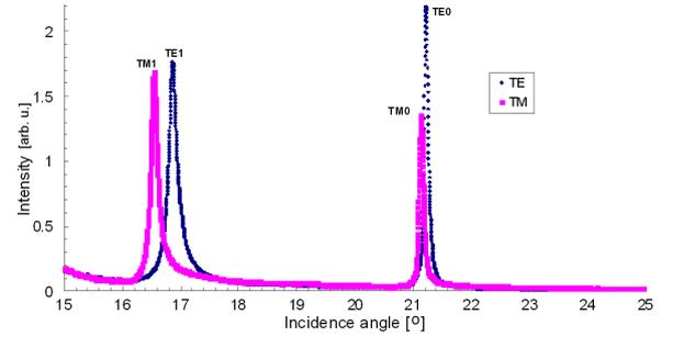
Fig. 1. Mode spectrum of the polymer waveguide SU8, obtained at rotational speeds of 2000 rpm.
