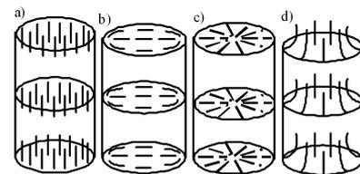
Fig. 1. Possible orientational configurations of nematic liquid crystal in a cylindric capillary with (a) planar (homogeneous, axial), (b) planar (transverse), (c) radial, (d) axial (splay) alignment.
