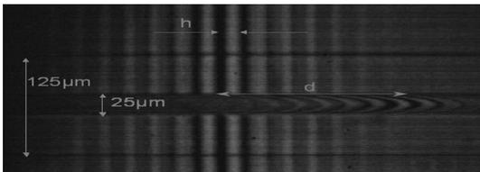
Fig. 5. Image of LC capillary ( $D = 25 \mu\text{m}$ ) with axial alignment configuration in optical interferometric microscope.
