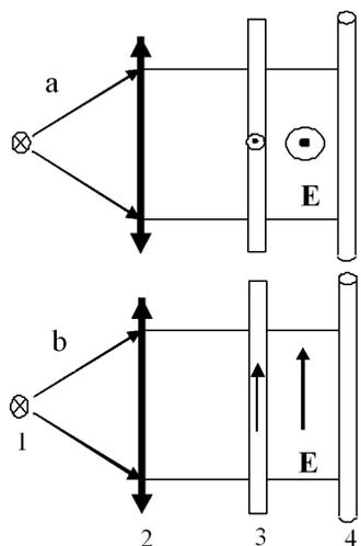
Fig. 2. Illumination schemes for planar (axial) (a) and planar (transverse) (b) alignment. 1 — UV lamp, 2 — collecting quartz lens, 3 — UV polarizer, 4 — sample.
