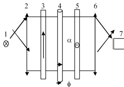
Fig. 3. Optical scheme of polarizing microscope with the sample positions during alignment inspection. 1 — light source, 2 — condenser, 3 — polarizer, 4 — samples, 5 — analyzer, 6 — objective, 7 — camera.
