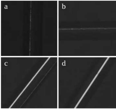
Fig. 4. The sample with planar LC configuration under the polarizing microscope. (a)  $\alpha = 0^\circ$ , (b)  $\alpha = 90^\circ$ , (c)  $\alpha = 45^\circ$ ,  $\phi = 90^\circ$ , (d)  $\alpha = 45^\circ$ ,  $\phi = 0^\circ$ ,  $\times 100$  magnification.
