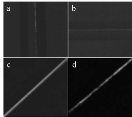
Fig. 6. The sample with transversal LC configuration under the polarizing microscope. (a)  $\alpha = 0^\circ$ , (b)  $\alpha = 90^\circ$ , (c)  $\alpha = 45^\circ$ ,  $\phi = 90^\circ$ , (d)  $\alpha = 45^\circ$ ,  $\phi = 0^\circ$ ,  $\times 100$  magnification.
