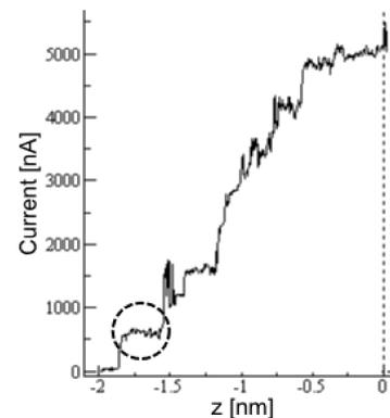
Fig. 1. Current vs. distance measured at a fixed bias voltage  $V = 10$  mV at 5 K. The last plateau (in the dashed circle) is at *ca.* 650 nA; this corresponds to a conductance of  $65 \mu\text{S}$ . For a single-atom contact the quantum conductance of approximately  $2e^2/h \approx 77 \mu\text{S}$  is expected. The exact value varies slightly due to the influence of the local atomic geometry.
