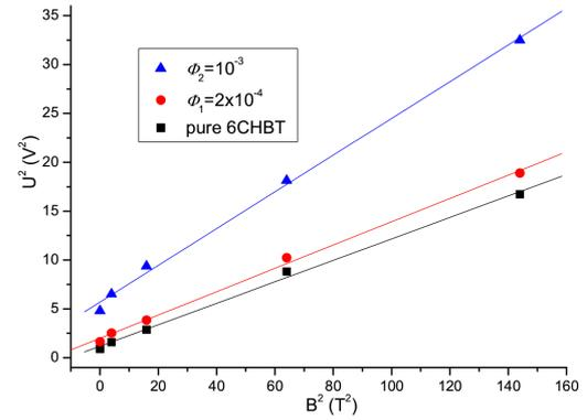
Fig. 4. Dependence of the critical electric fields on the bias magnetic field for pure 6CHBT and 6CHBT doped with gold particles with volume concentration  $\phi_2 = 2 \times 10^{-4}$  and  $\phi_2 = 10^{-3}$ . The solid lines represent the best linear fit to Eq. (1).
