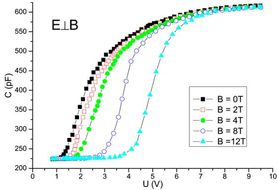
Fig. 2. Capacitance dependence of 6CHBT doped with gold particles with volume concentration  $\phi_1 = 2 \times 10^{-4}$  on electric field measured at different bias magnetic fields.
