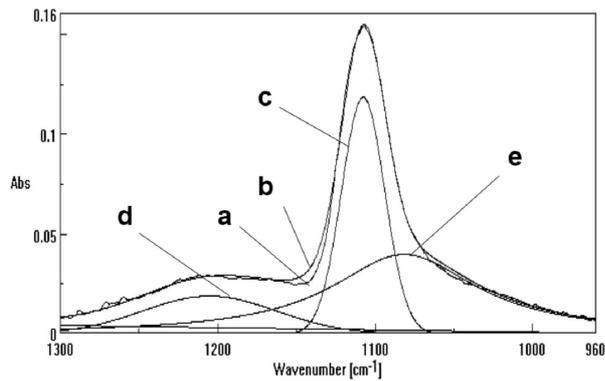
Fig. 4. Deconvolution of IR absorption band at  $1107\text{ cm}^{-1}$  (a, b) on different sub-bands (c, d, e) for Cz-Si:N sample pre-annealed for 10 h at 923 K under 1.1 GPa and finally processed for 5 h at 1270 K under 1.1 GPa. See Fig. 3 caption for explanation of deconvoluted sub-bands.
