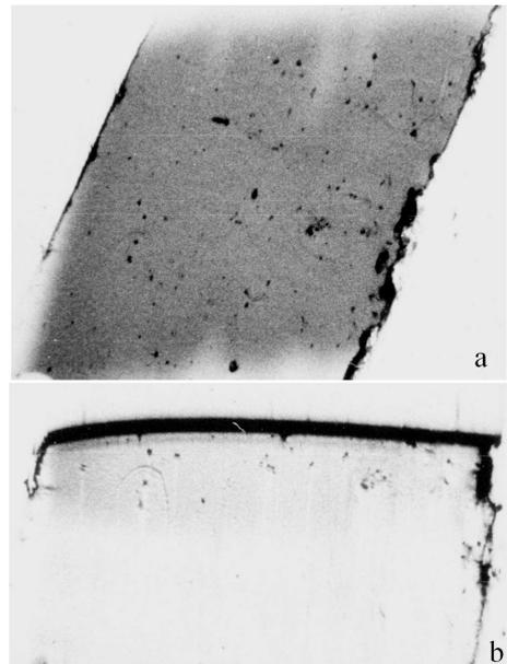
Fig. 6. White beam projection (a) and section (b) topographs of Cz-Si:N processed for 5 h at 1400 K under 0.3 GPa. Width of reproduced area equals to 8 mm.
