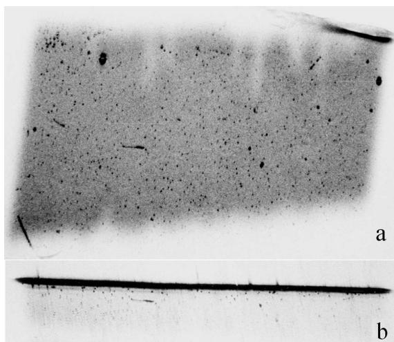
Fig. 5. White beam projection (a) and section (b) topographs of Cz-Si:N processed for 5 h at 1400 K under  $10^7\text{ Pa}$ ; after processing  $c_{\text{O}} = 8.5 \times 10^{17}\text{ cm}^{-3}$ . Width of reproduced area equals to 8 mm.
