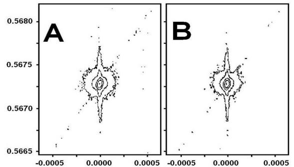
Fig. 2. XRRSM's of Cz-Si:N samples pre-annealed for 10 h at 923 K under  $10^5$  Pa (A) or 1.1 GPa (B) and finally processed for 5 h at 1270 K under 1.1 GPa. Axes are marked in  $\lambda/2d$  units ( $\lambda$  — wavelength,  $d$  — interplanar distance).
