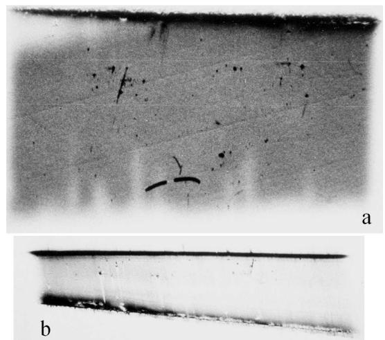
Fig. 7. White beam projection (a) and section (b) topographs of Cz-Si:N processed for 5 h at 1400 K under 1.1 GPa; after processing  $c_{\text{O}} = 5 \times 10^{17}\text{ cm}^{-3}$ . Width of reproduced area equals to 8 mm.
