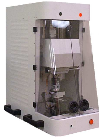
Fig. 6. CETR universal tribometer in the UMT-2 configuration.
