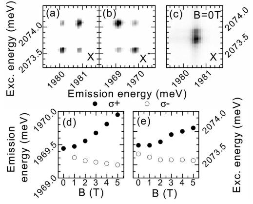
Fig. 4. (a) X and (b) X<sup>-</sup> PLE maps measured in  $B = 4$  T. (c) PLE map of X without magnetic field. Zeeman effect in (d) emitting and (e) absorbing QD. Data from Ref. [30].
