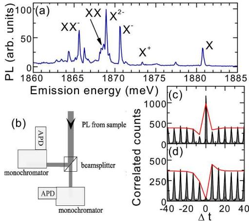
Fig. 1. (a) PL spectrum of a typical quantum dot. (b) Scheme of HBT detection setup used in correlation experiments. (c) Cascade-like correlation histogram between neutral biexciton and exciton. (d) Asymmetric correlation histogram between charged and neutral exciton.
