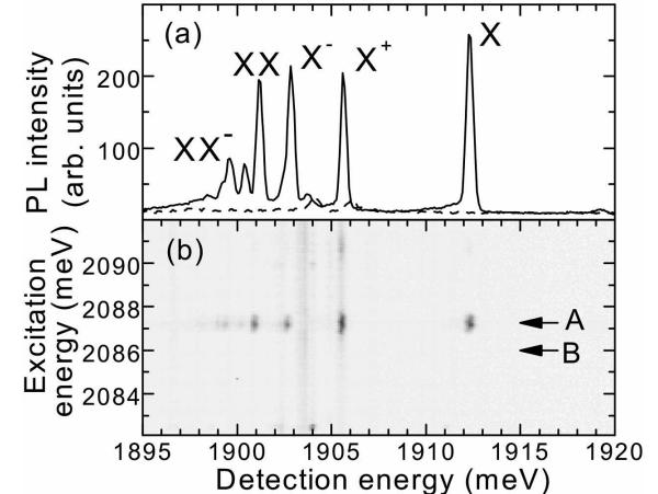
Fig. 3. (a) PL of a single QD measured under resonant excitation (solid line) and after detuning by 1 meV (dashed line). (b) Corresponding PLE map of the QD. Energies of the presented PL spectra are denoted by A and B. Data from Ref. [30].
