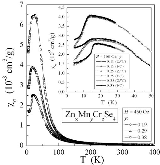
Fig. 2. The dc mass susceptibility  $\chi_\sigma$  vs. temperature  $T$  for polycrystals with  $y = 0.19, 0.29$  and  $0.38$  of the  $\text{Zn}_x\text{Mn}_y\text{Cr}_z\text{Se}_4$  spinel system recorded at  $H = 450$  Oe. Inset: ZFC and FC dc mass susceptibility  $\chi_\sigma$  vs. temperature  $T$  recorded at  $H = 100$  Oe.
