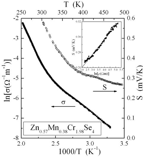
Fig. 1. The electrical conductivity ( $\ln \sigma$ ) vs. reciprocal temperature  $T^{-1}$  and thermopower  $S$  vs. temperature  $T$  for  $\text{Zn}_{0.57}\text{Mn}_{0.38}\text{Cr}_{1.98}\text{Se}_4$ . Inset: thermopower  $S$  vs. electrical resistivity ( $\ln \rho$ ). A linear regression is marked by a solid line.
