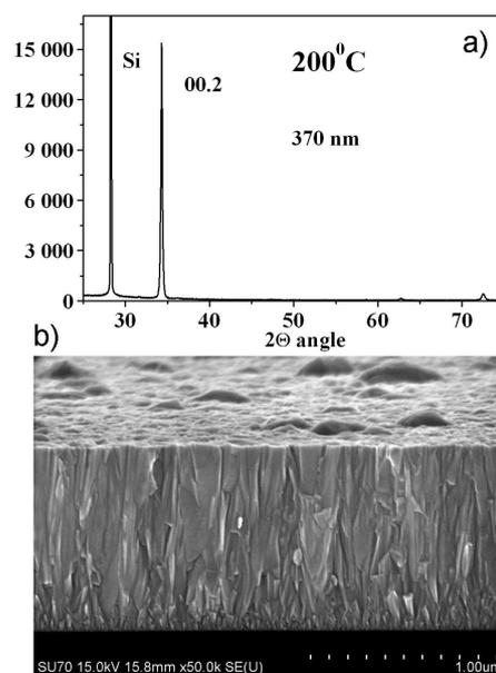
Fig. 1. (a) The XRD spectrum of the polycrystalline ZnO film with  $c$  axis perpendicular to the surface. (b) The SEM image of a low temperature polycrystalline ZnO film.
