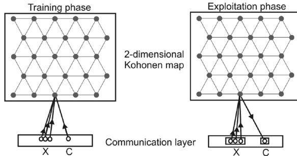
Fig. 2. Schematic of SSOM architecture (communication layer is connected to all nodes in Kohonen map — for the simplicity connections are drawn just to one node).
