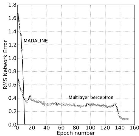
Fig. 4. The dependence of the RMS error of multilayer perceptron and the MADALINE network in the subsequent learning epochs.
