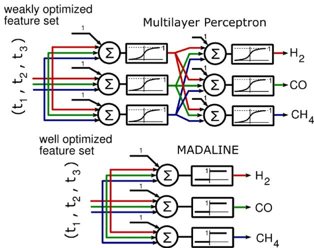
Fig. 3. The structure of the classifiers for unoptimized and optimized secondary feature spaces.
