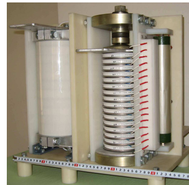
Fig. 4. 25 kV microsecond RSD based switch with 300 kA peak current and 30 kA/ \mu s current rise rate.
