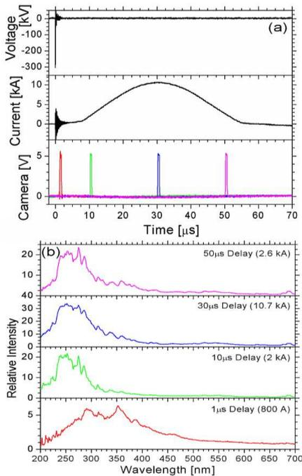
Fig. 2. (a) Typical high current volume breakdown waveforms and camera gates. (b) Optical emission spectra of volume breakdown at 2.3 bar of SF<sub>6</sub> [2].
