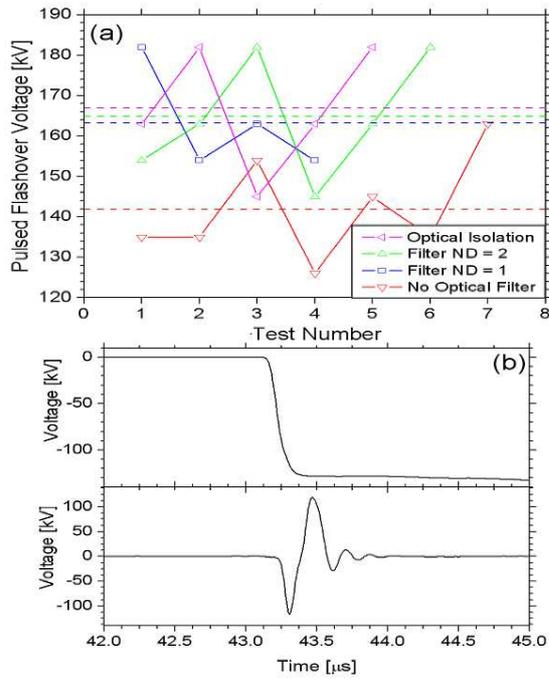
Fig. 4. (a) Flashover voltage of a 24 mm gap across Lexan with varying levels of light attenuation from a  $\sim 10$  kA volume discharge. The dashed lines represent the mean value for each data set. (b) Voltage waveforms measured with capacitive divider in 50  $\Omega$  transmission line; top: no flashover, bottom: flashover.
