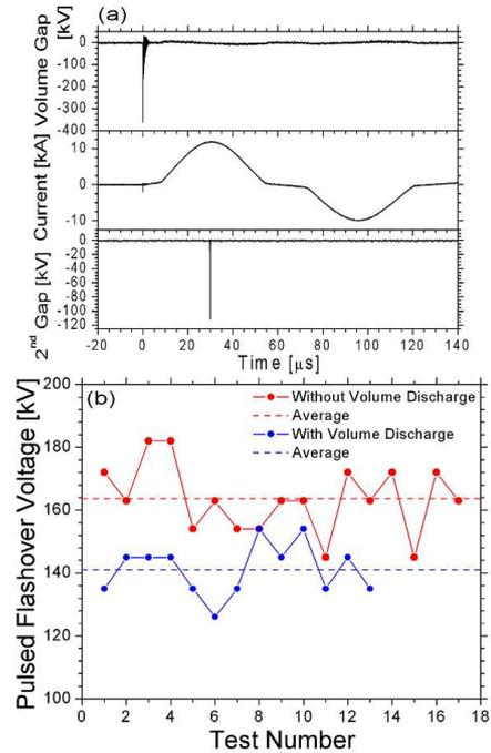
Fig. 3. (a) Voltage and current waveforms illustrating the relative timing of the high current volume gap and the secondary surface flashover gap. (b) Pulsed voltage necessary to flashover the secondary gap both with the high current volume discharge (bottom curve) and without (top curve).
