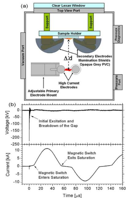
Fig. 1. (a) Side view of the chamber configured for high current discharge / surface flashover interaction testing. Diagram illustrates the relative position ( $\Delta d \sim 7$  cm) of the primary volume and secondary surface flashover gaps. (b) Typical volume breakdown waveforms at 3.7 bar of SF<sub>6</sub>.
