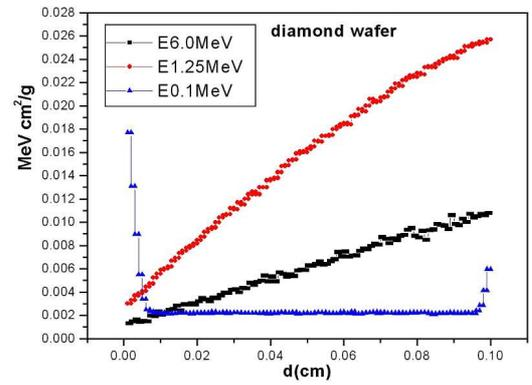
Fig. 3. Deposited energy in layer of diamond wafer.
