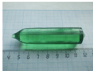
Fig. 1. An "as grown" YAG:V single crystal obtained by the Czochralski method.
