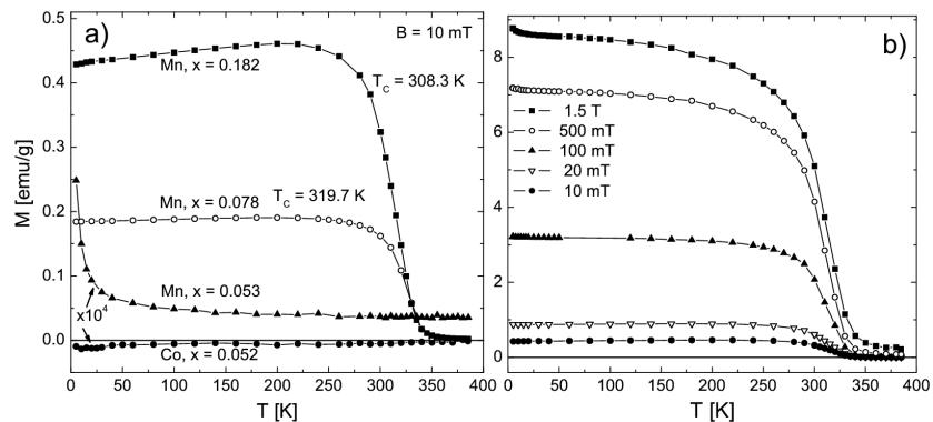
Fig. 1. The magnetization  $M$  as a function of temperature: (a) measured for the  $Zn_{1-x}(Mn,Co)_xGeAs_2$  samples with different chemical compositions (labels), and (b) measured using different applied magnetic fields (legend) for the  $Zn_{0.818}Mn_{0.182}GeAs_2$  sample.
